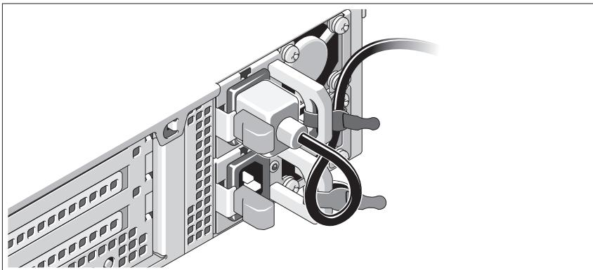
Bend the system power cable into a loop as shown in the illustration and secure the cable to the bracket using the provided strap. Plug the other end of the power cable into a grounded electrical outlet or a separate power source such as an uninterrupted power supply (UPS) or a power distribution unit (PDU).
